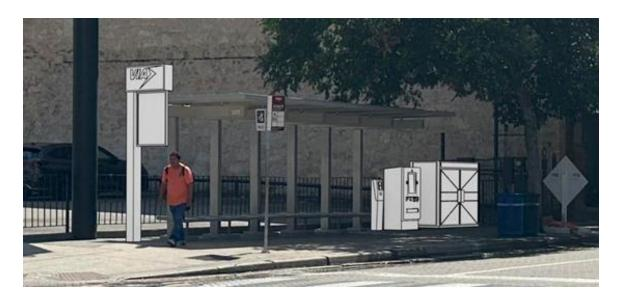
**Figure 3:** Example station rendering, side-running configuration in downtown (VIA 2024). This configuration is located on one side of the street along the curb. These stations would include a canopy. In some cases, the station platform would be raised and include a ramp at one or both ends.
