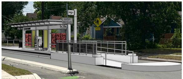
**Figure 5:** Example station rendering, center-running configuration on a road with two-way traffic outside downtown (VIA 2024). This configuration is located at the center of the street, allowing service from both sides. These stations would include a canopy, the station platform would be raised, and ramps would allow access at one or both ends.
