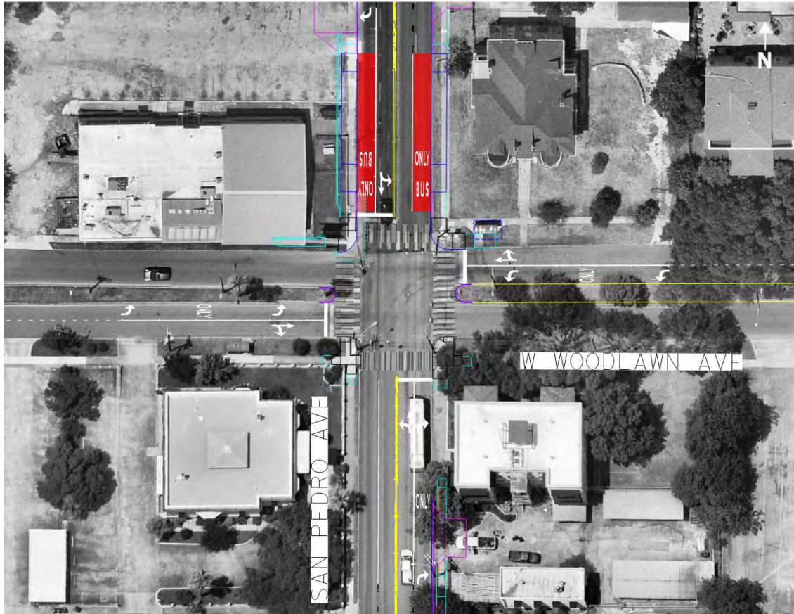
Figure 25: Woodlawn at San Pedro Intersection - After Mitigation
