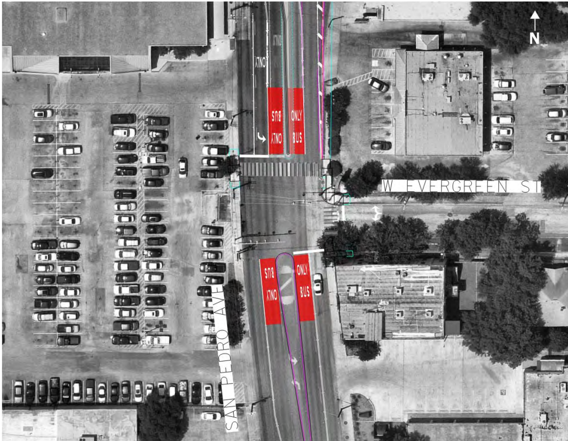
Figure 27: Evergreen St at San Pedro Intersection - After Mitigation
